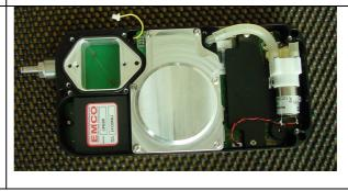
Once you reach the last stage above, you should see a white deposit on the wire. Take a fine artist's paintbrush and wipe the corona wire VERY GENTLY with it. The wire is very thin and if mechanically stressed, it will break. Reassemble the instrument in reverse order. When reinstalling the counterelectrode, check that the o-Ring is placed nicely in its groove.
