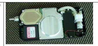
Now remove the 4 hex screws holding the counterelectrode in place; lift off the counterelectrode and optionally disconnect it from the yellow cable, to get it out of the way.
