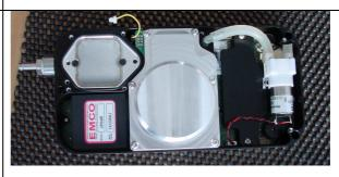
Remove the two black hex screws holding the wire-mesh screen in place and GENTLY remove the wire mesh screen. Be careful not to bend the wire mesh, this would affect the calibration!
