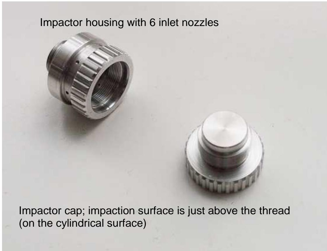
The impactor has to be cleaned regularly after use; open it by removing the cap, and wipe the smooth surface below the thread to screw the cap into the impactor housing. From time to time, the 6 impactor nozzles in the housing should be cleaned; the easiest way to do this is to use an ultrasonic bath.
